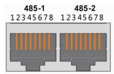
With dual RS485 interfaces, the default baud rate is 9600bps. If you need to communicate the batteries in parallel with the monitoring device or inverter, you need to connect each battery with RS485-1 and RS485-2 ports, so the host battery can read the information of each battery.
